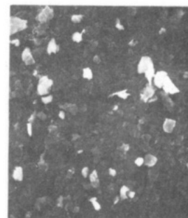
Figure 1. Effect of ultrasonic irradiation on surface morphology of 75-μm Cu powder. Note the increase of magnification of these scanning electron micrographs from left to right. SEMs were obtained on a Hitachi S-800 microscope.
